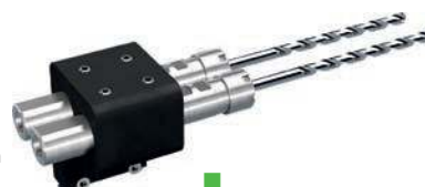
Tool block with 2 bores to accept drill holders for deep drilling. Mounts on the left side of the counter spindle. Maximum drilling length: 160 mm. Fitted with connection for high pressure coolant.
