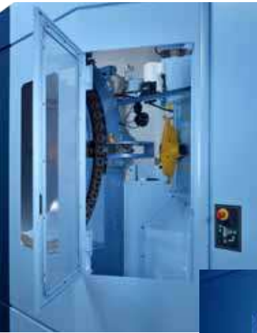
The ATC front door provides easy access for maintenance.
