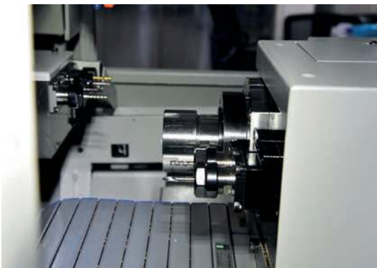
Rotating tools next to counterspindle (option)
