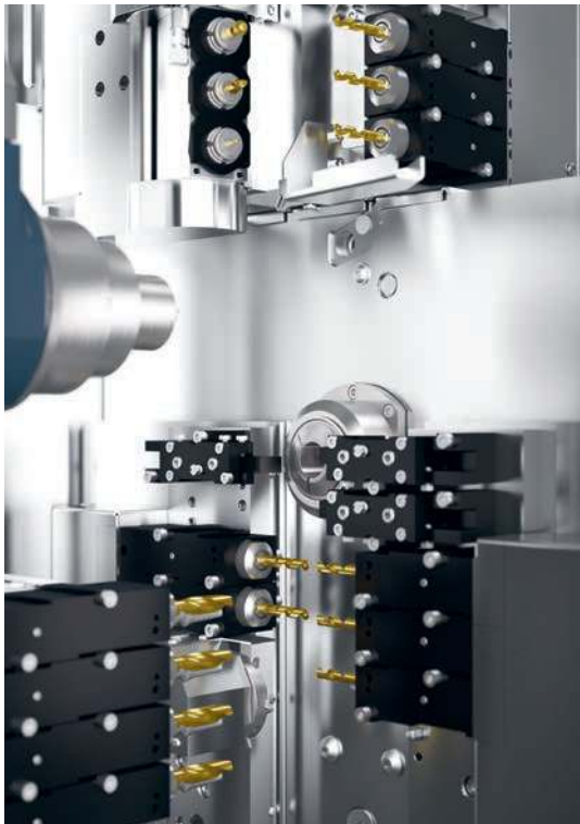
EvoDECO 16/10: 10-axis kinematics
