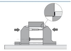
Thanks to its own expanding screw, GENIUS can clamp workpieces up to 200 mm with just one set-up.
